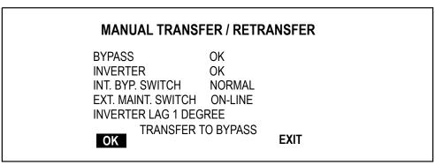
Figure 32 Manual transfer / retransfer screen when transfer is not allowed
